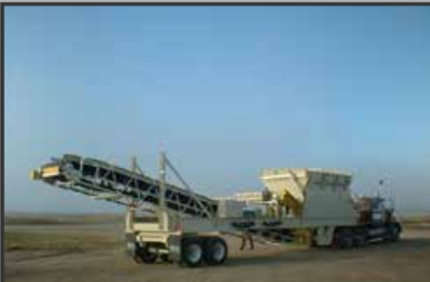
New 4242 HD Belt Feeder tandem axle, brakes & lights, hyd. grizzly adjustable 16" spacings P.O.R.
