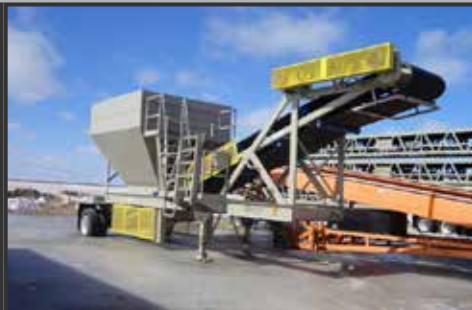
New 30 Yd. Surge Bin single axle, brakes & lights, 42" discharge belt c/w 40 HP electric motor, 100 ft cord pkg. inspection platform, safety shut down switch. P.O.R.
