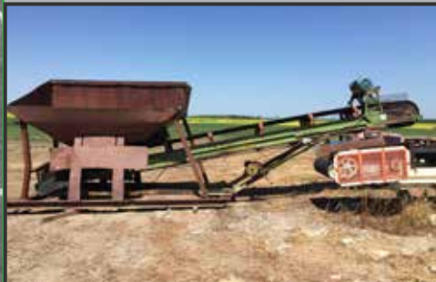
Skid Feeder c/w 24" discharge belt, 25 HP electric motor, 5 ft 6" discharge hght. electrical control box $9,500
